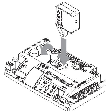
• Check that the side signalling led goes on (module enabled and ready for communication). Proceed to associate the WiFi network generated by the module (e.g. SSID: comunelloWiFi\_ONE#04081230) to your mobile device. From the configuration menu of your device, search for the available WiFi networks and select the network "comunelloWiFi\_ONE#..." (the numerical code after the # character is variable).
